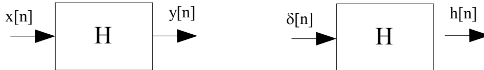
Figure 1: Input-output relationship for a digital filter produces the impulse response when the input is an impulse function.
